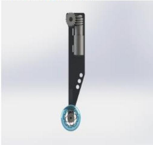
Figure 3: Stabilization Legs Deployed
