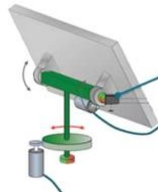
**Figure 2: Base with 2 axes of rotation using two 9g servos**
